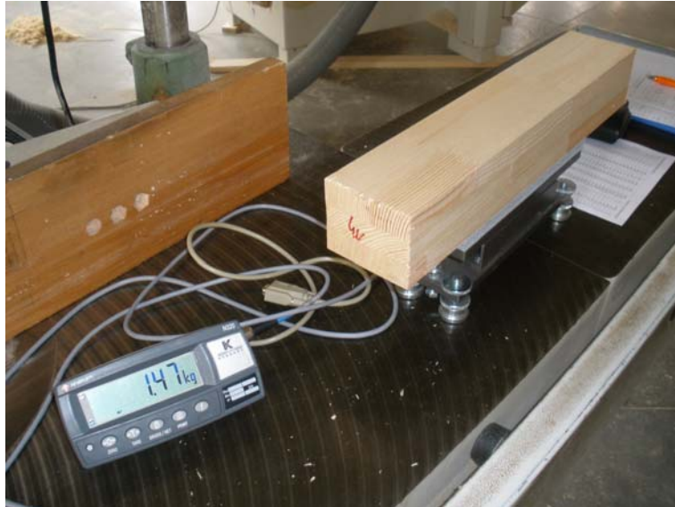
Figure 3: Measurement of mass after cutting to length
