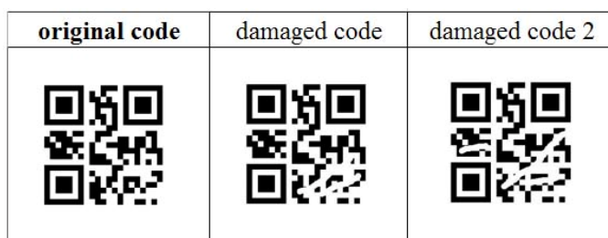
Figure 2. Image of the generated code which by scanning leads to the following text: “QR 2D kod”, and the same code with simulated damage
