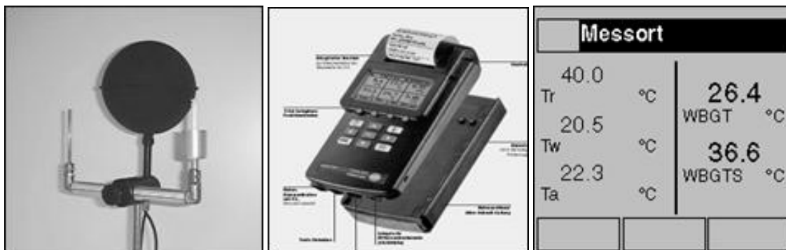
Figure 4: WBGT sensor, measurement, display
