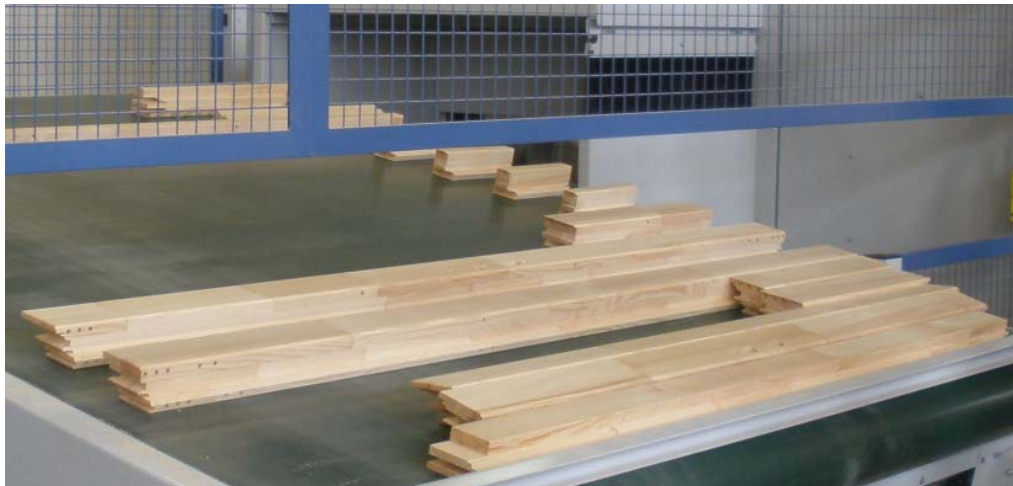
Figure 4: Frame parts after profile machining
