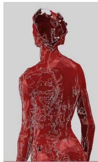
Figure 5: Reducing number of polygons and repairing the mesh in programme ATOS
