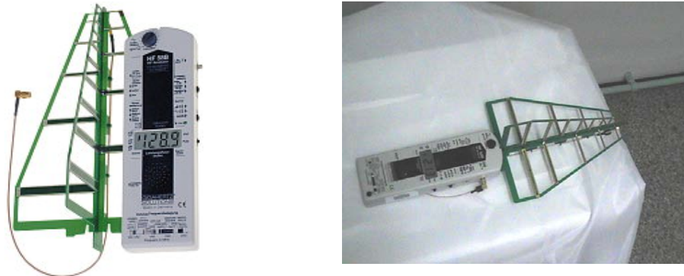
Figure 1: HF 58B Electro smog measuring set-up
