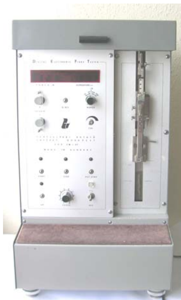
Figure 3: Fm-27 type electronic single fibre tensile tester
