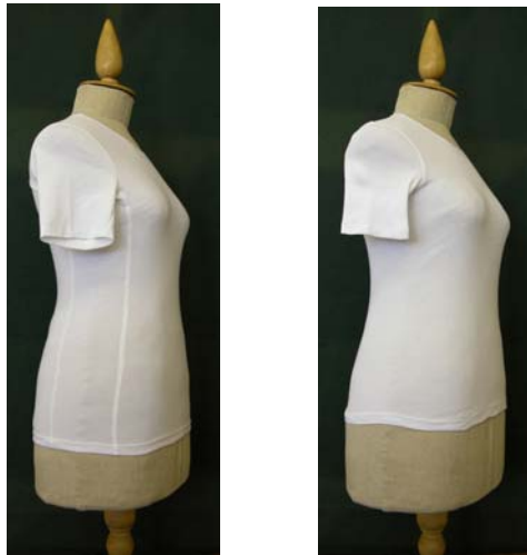
Figure 8: T-shirt with overlapping stitching and without stitching
