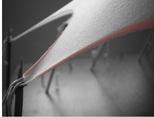
Figure 5: Edge without a perimeter cable
