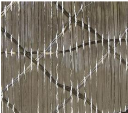
Stitched unidirectional fabric, 0 direction
