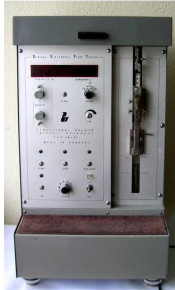
Figure 1. Fm-27 type electronic tensile strength tester for filaments
