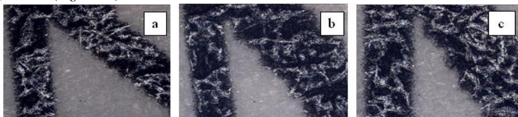
Figure 10: Videomicroscopic line image of the artificially created line (left) and the original graphic (right) with the use of a. CorelDRAW program, b. Adobe PhotoShop, c. Adobe InDesign
