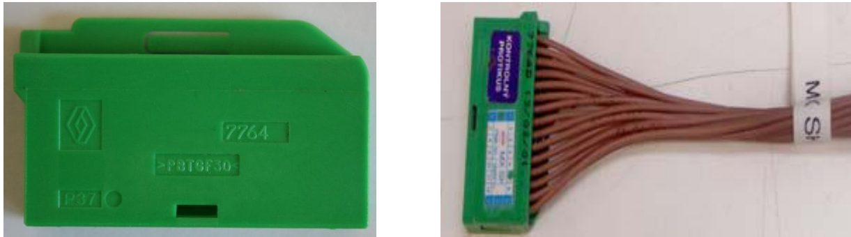
Fig. 11 The molding made from PBT material and his using in automobile
