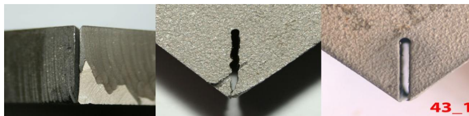
Figure 7: The cutting gap of the sample 43.1 – view form the right to left upper, lower and front ones
