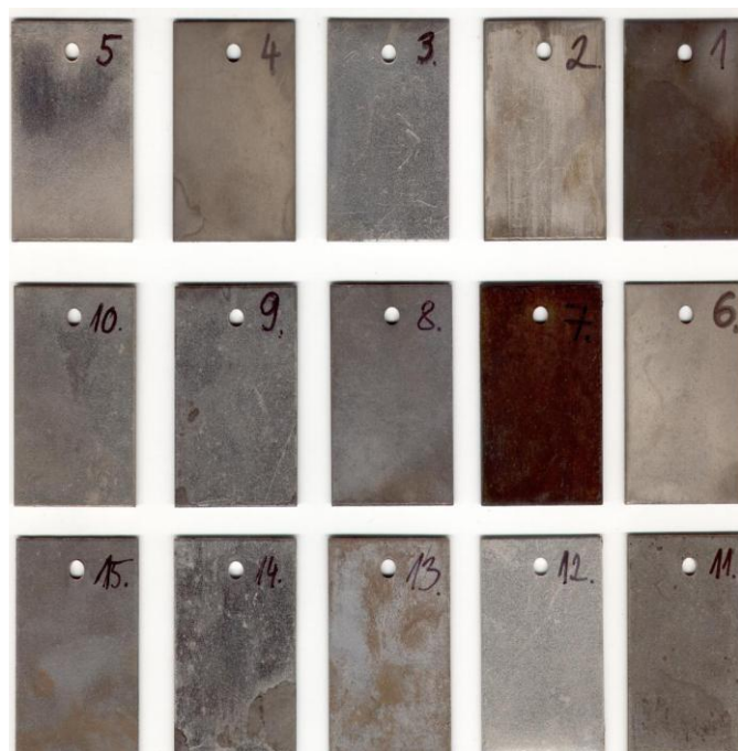
Figure 2: Samples after chemical nickeling of the planned experiment
