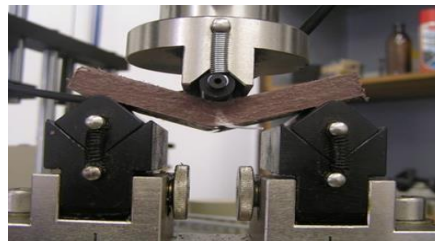
Figure 14. The detail of the bending test
