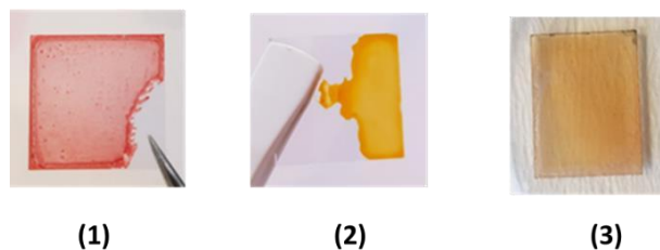
Figure 3. Typical drop-casted samples of complexes 1 , 2 , and 3 on the ITO slides, applied in improved electrocatalysis to generate \text{O}_2 [23], [24].
