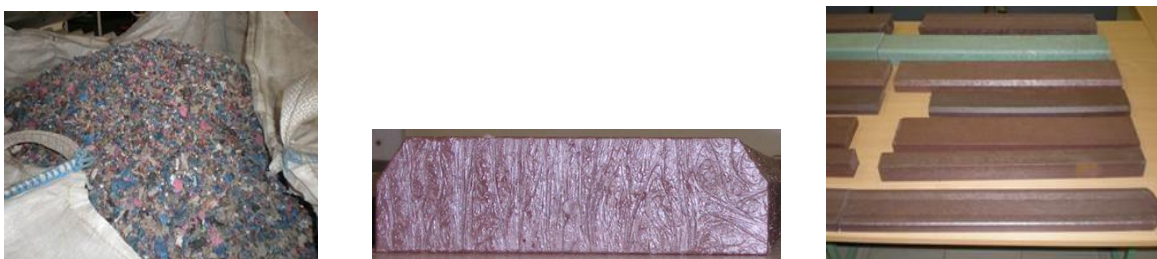
Figure 12. Supplied plastic sorted semi- product and final plastics boards from recycled material
