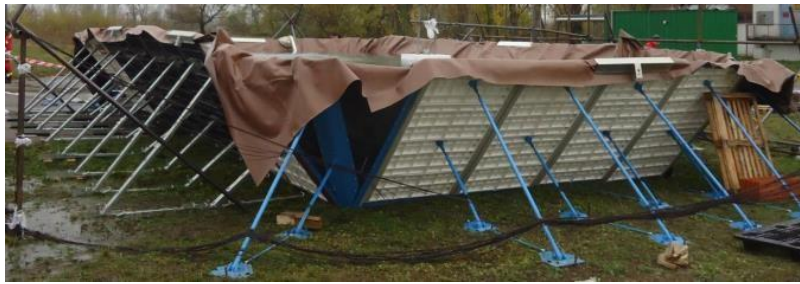
Figure 10. Modular flood barrier structure – test basin at TOP 2016 [7]
