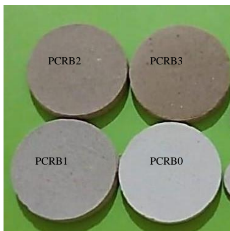
Figure 2. Photos of the ceramic samples sintered as function of SBWs addition sintered at 1200°C.
