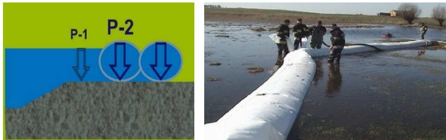
Figure 3. system with one or two cylinder plastic foils barriers [4, 6]
