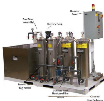
Figure 4. The Closed Loop Filtration System Model Model #CLS-138 [5]
