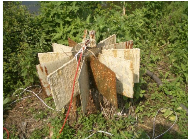
Figure 16: Store the electrode and its condition after the experiment on the lake
