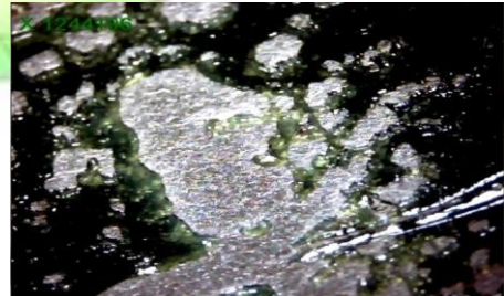
Figure 18 Detail of degreasing of lubricant by USB microscope
