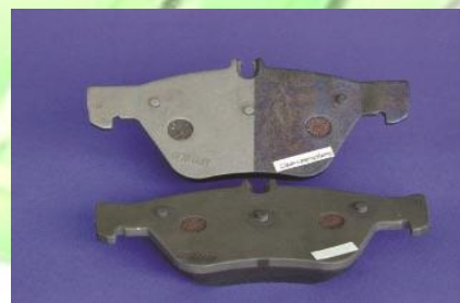
Figure 8 Brake pads before and after laser cleaning.[9]
