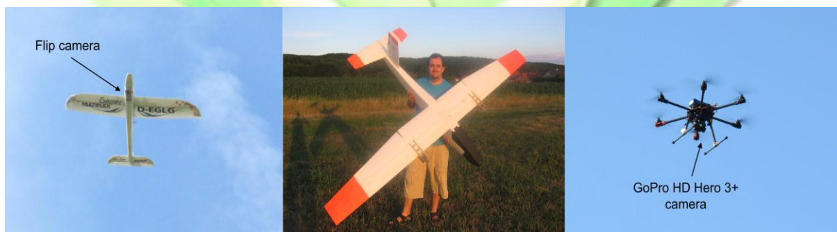
Fig. 5: The UAVs used in the experiments: MULTIPLEX Easy Star (left), STYROMAN Smile (centre) and TAROT 690S (right)
