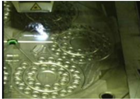
Figure 9 Cleaning of an injection mould [10]
