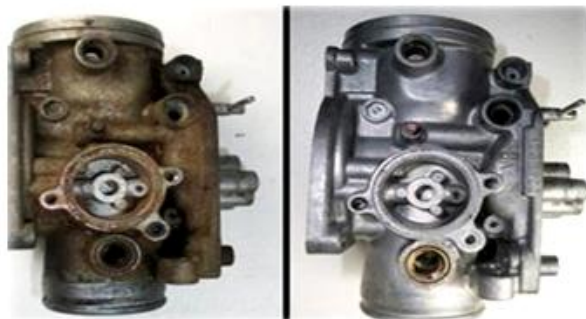
Figure 2 Example of US cleaning of product before and after cleaning
