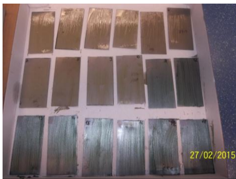
Figure 10 Tested materials KOSMALT 190
