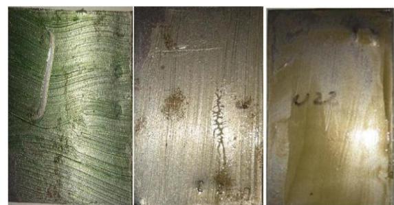
Figure 11 Tested samples No. 14, 7, 29 before degreasing by laser cleaning
