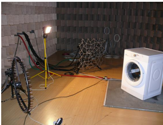
Figure 3 Noise visualization measurements in anechoic chamber by the acoustic camera and noise inspector
