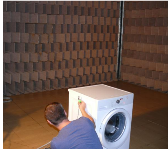
Figure 4 Noise visualization measurement in anechoic chamber by the combined sensor microflown
