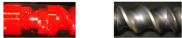
Figure 6 The extrusion screws before and after cleaning operation [7]
