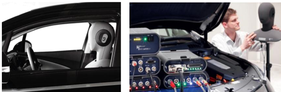
Figure 1: Measurement of psychoacoustic parameters in an automobile interior
