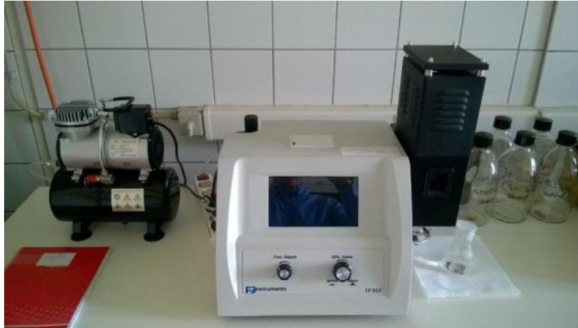
Figure 3. FP910 (PG Instruments) Flame Photometer
