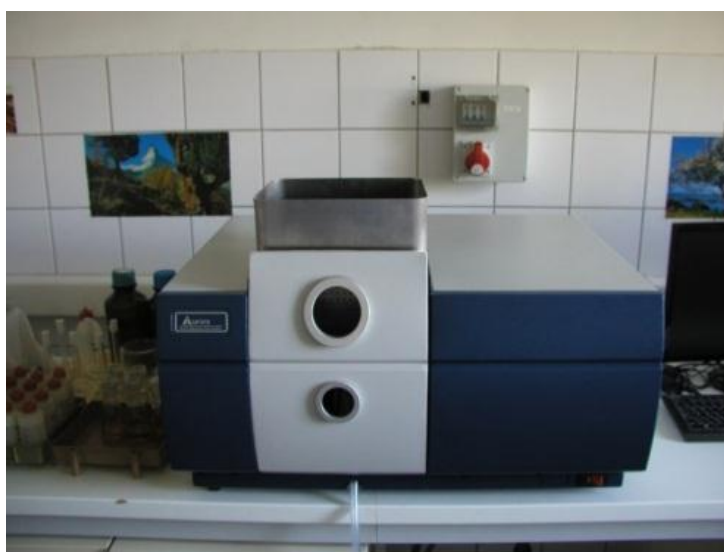
Figure 2. AURORA AII200 Atomic Absorption Spectrometer
